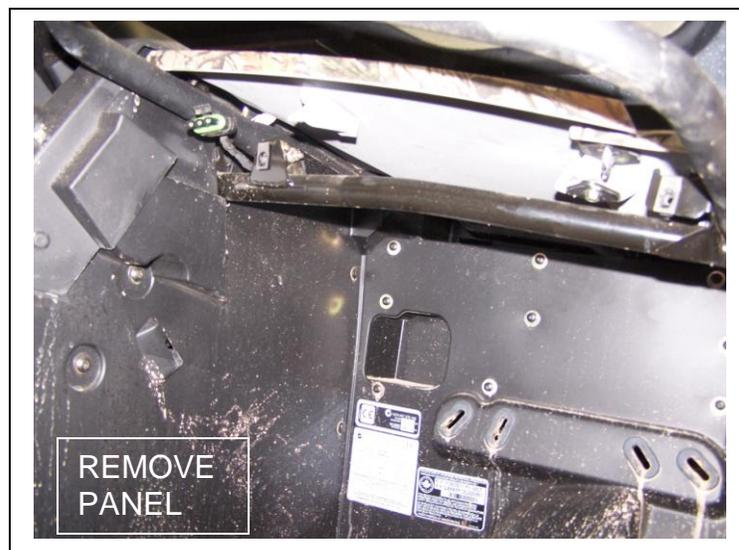
5) Remove (2) Torx screws and (2) retainers from center dash switch console and gently set it aside to gain access to dash interior. **Note: Switches need not be disconnected.**
