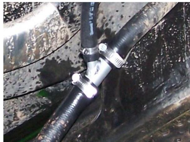
9) Repeat step 8 on radiator hose located above driver's side front wheel. Note Y-Adapter orientation. Attach and route longer heater hose through center of vehicle and out through passenger side "foot well" area. Elevate hose and keep together with previously installed heater hose. Using 2 or 3 zip ties, secure hoses to vehicle to prevent chafing.
