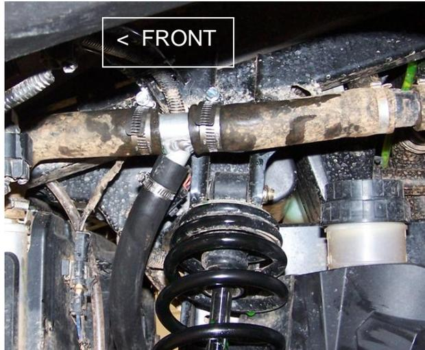
10) Keeping hose ends elevated, feed them through 1" holes of inner side panel and pinch them to prevent coolant loss. Set the hoses down into the passenger seat area in order to reinstall the side panel in it's proper location. Note: Continue to pull hoses through panel ensuring they are not binding and/or kinking. Reinstall OEM hardware onto inner side panel.
